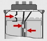
Patented 3-Phase Disconnection at internal over-pressure
