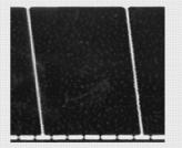
Unique Film Design with Segmented Metallization
